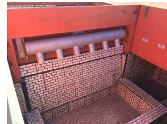
Figure 3: Ceramic lined pulping box
