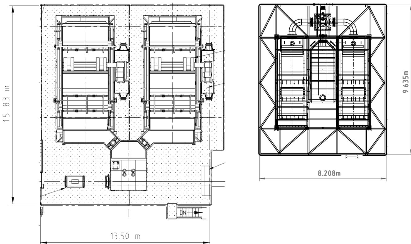
FIG 3 – Size comparison between conventional cyclone overflow trash screens - left (Lycopodium 2011) and HFLS - right.
