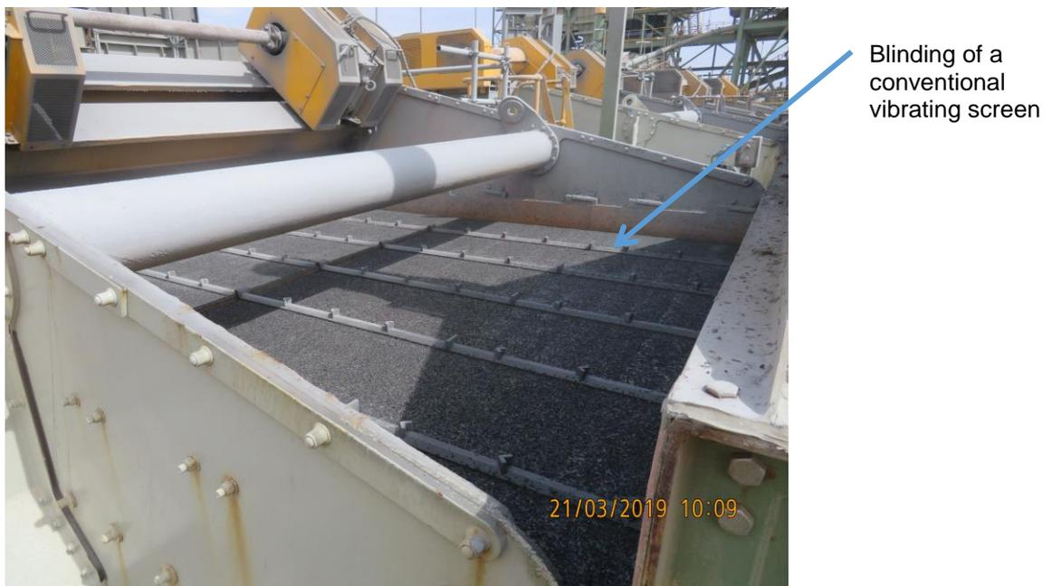
FIG 4 – Blinding of conventional screens greatly reduces screen open area resulting in lower screening capacities.
